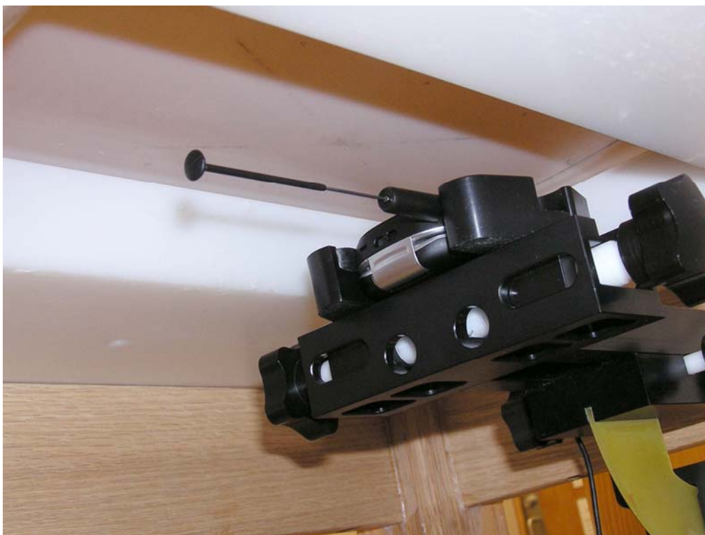
Figure 12. Phone Against the Flat Phantom with antenna extended
