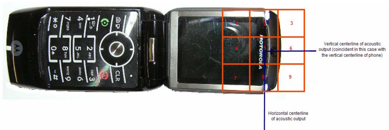
Figure A6-2. Phone Open - Orientation of Wireless Device and Measurement Plane
