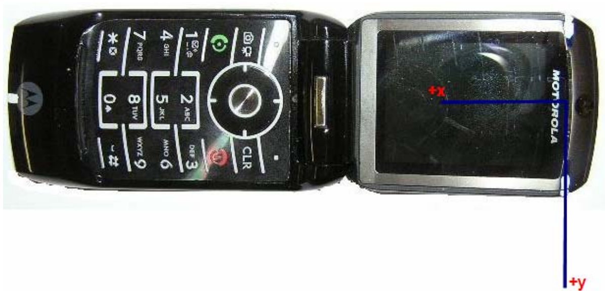
Figure A4-2. Phone Open – Coordinate Axis for T-coil Measured Point Location
