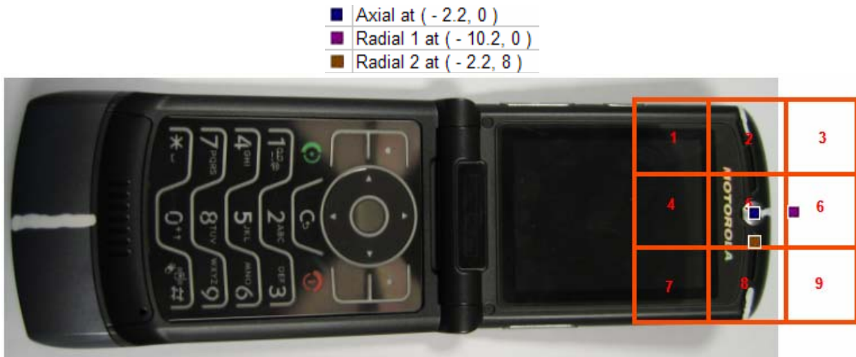
Figure A4-3. Phone Open – Location of Measured Points for T-coil – 5cm x 5cm grid for Near Field Measurements
