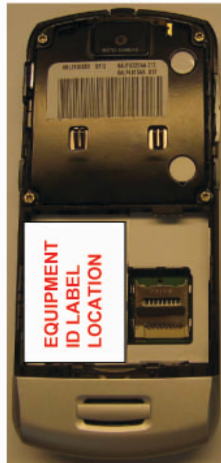
BACK OF PHONE WITH BATTERY COVER REMOVED
