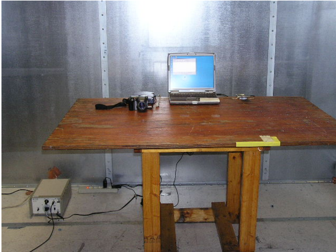
AC Line Conducted Emissions Measurement Setup. (Representative Photo- Not Actual Phone Tested)
