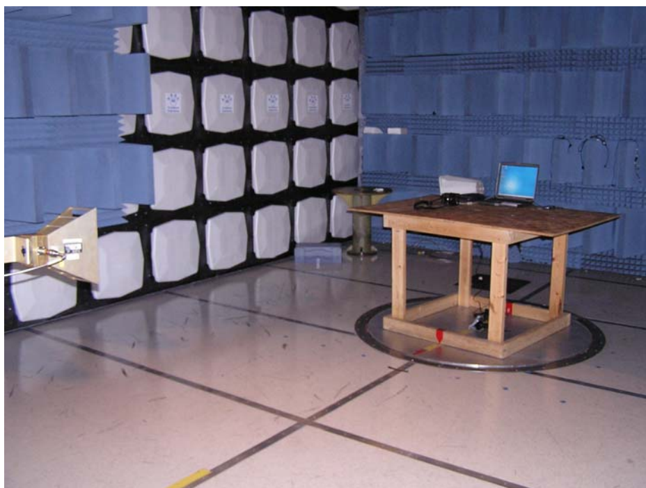
Figure 2. Part 15 Radiated Emissions Measurement Setup
