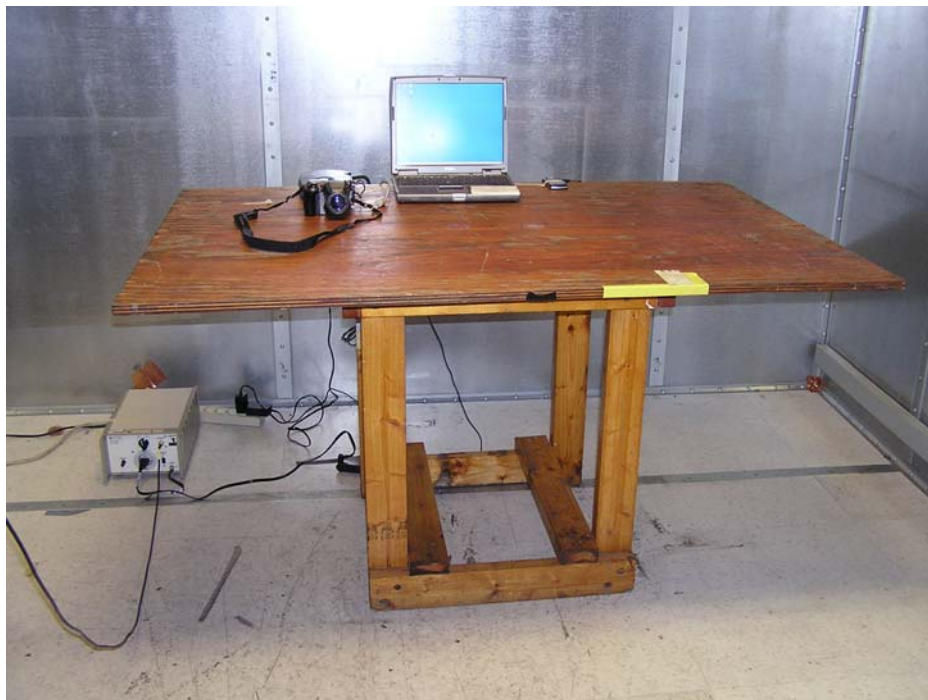
Figure 1. AC Line Conducted Emissions Measurement Setup
