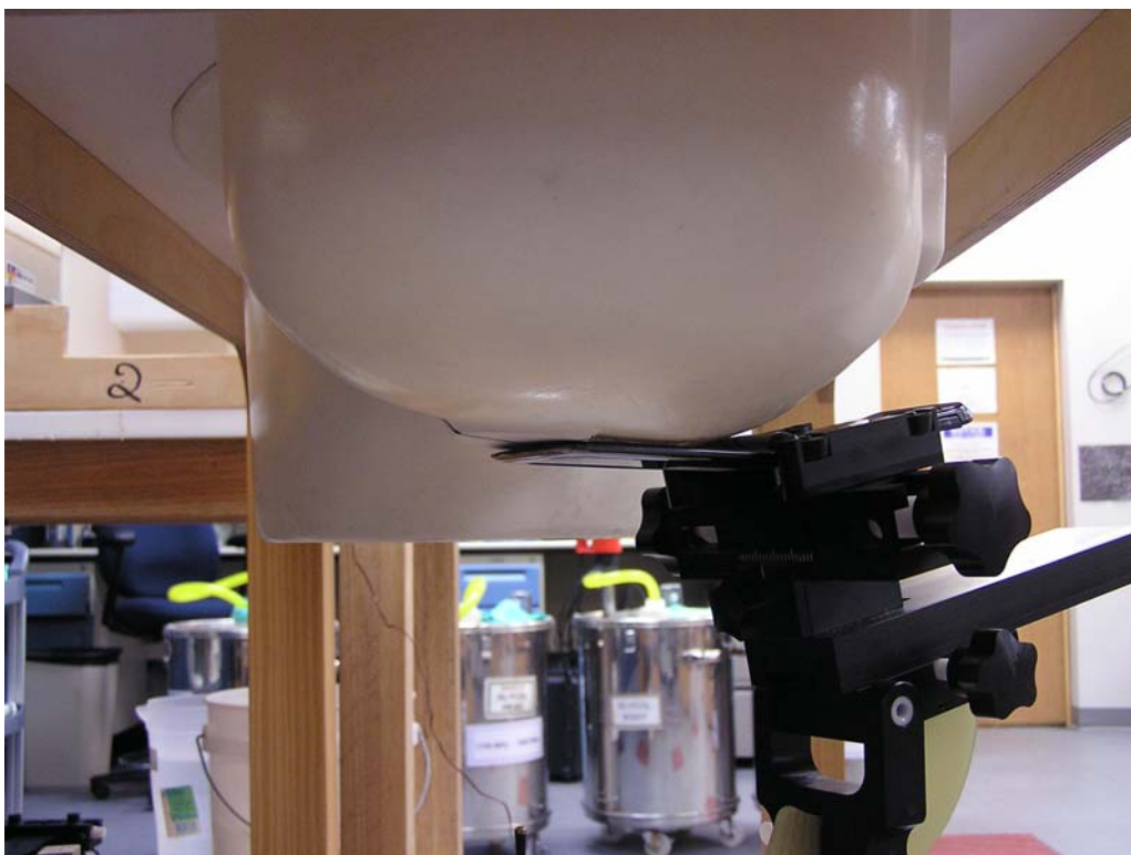
Figure 4 – Transceiver against head, Cheek Touch position
