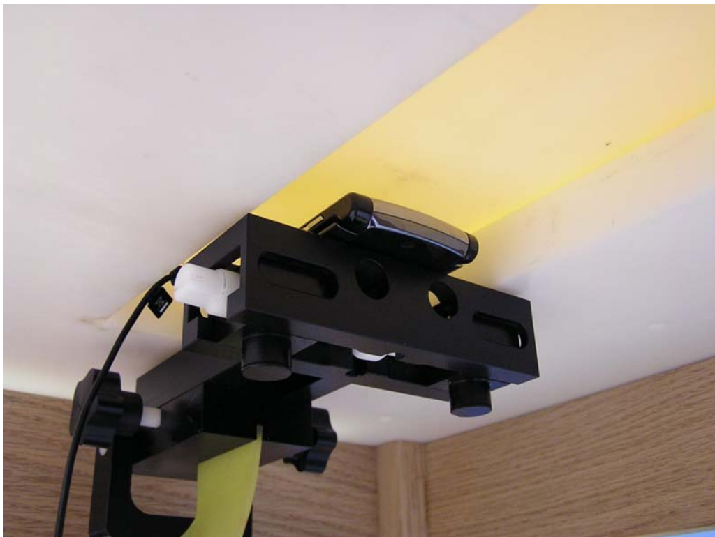
Figure 8 – Transceiver against body, Back of Phone 15 mm from Phantom position
