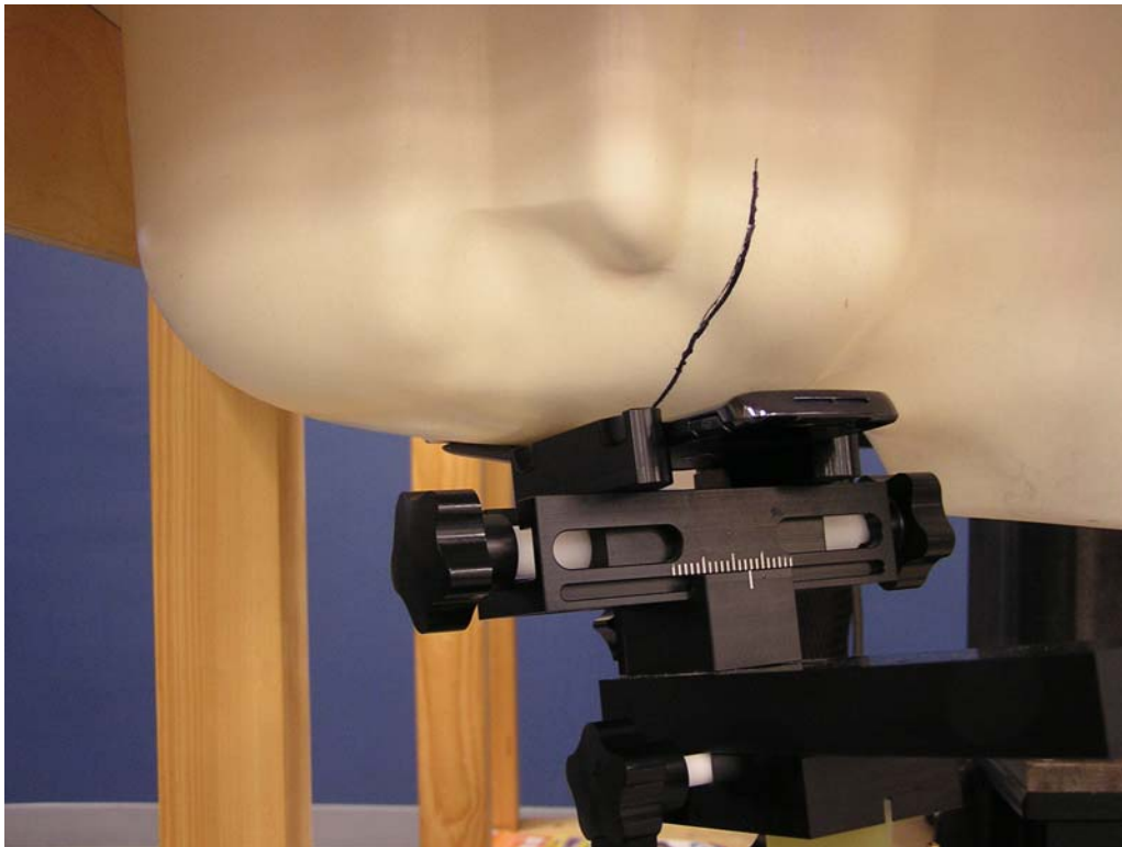
Figure 3 – Transceiver against head, Cheek Touch position
