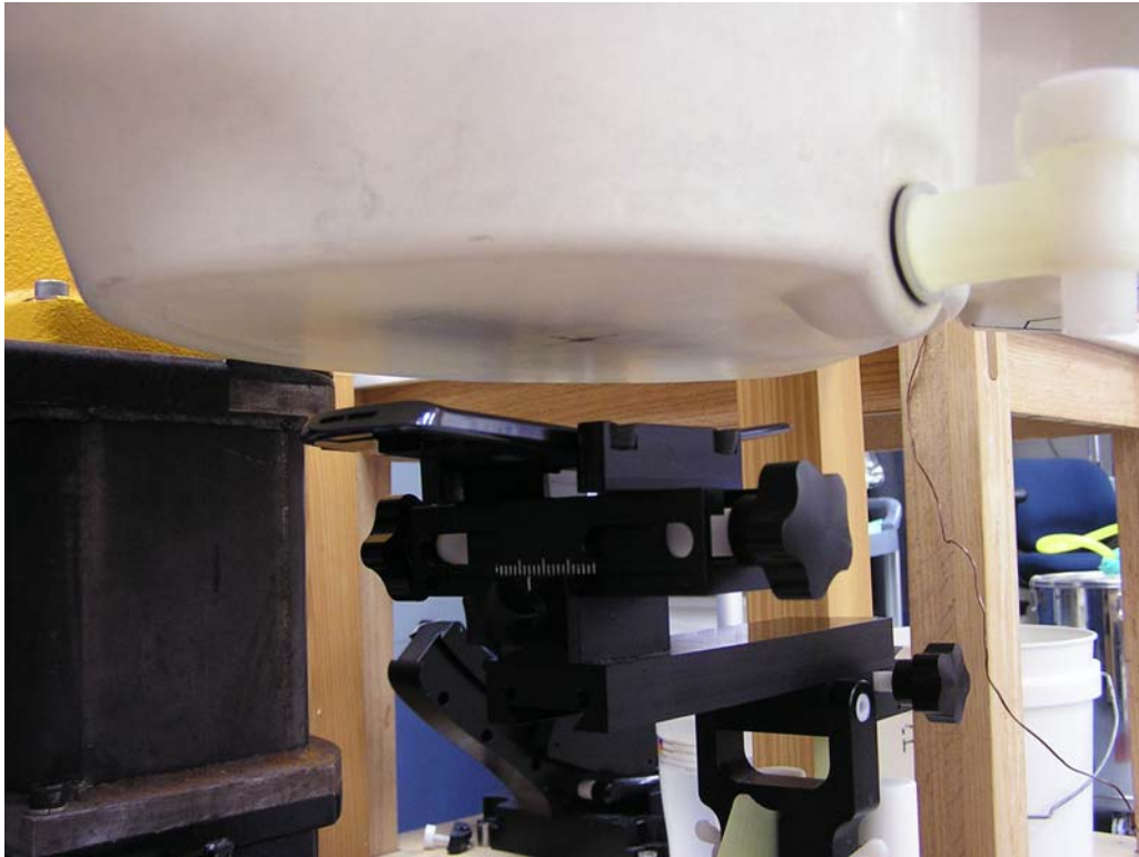
Figure 7 – Transceiver in Face Dispatch position, 25 mm from Phantom
