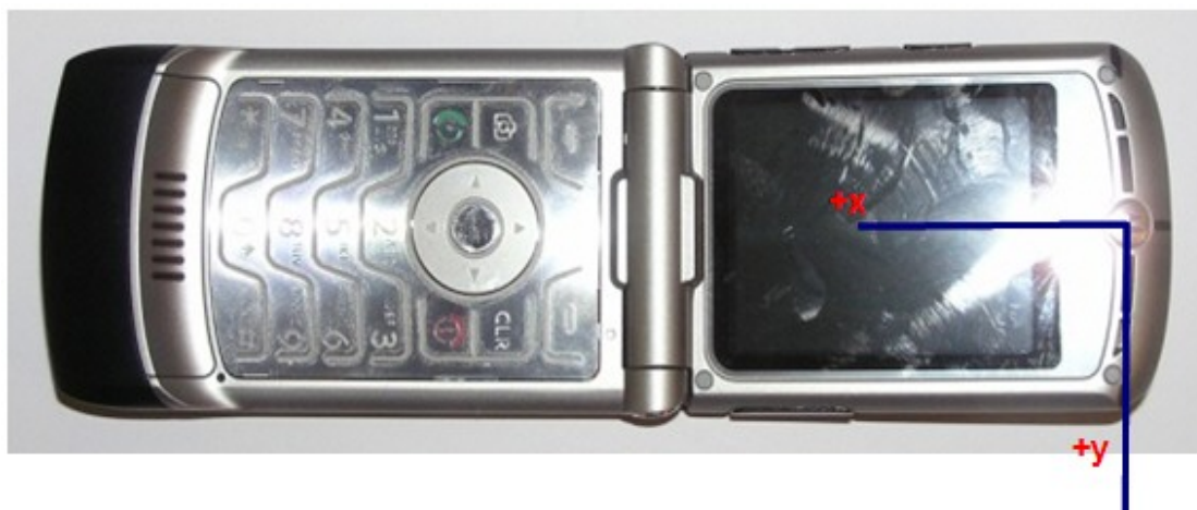
Figure A4-4. Coordinate Axis for T-coil Measurements
