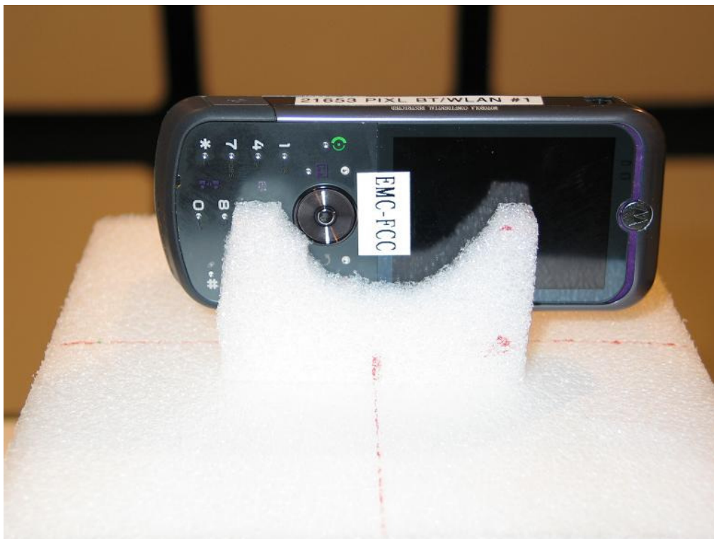
21653-1, IHDT56JT1 placed in test position Y
