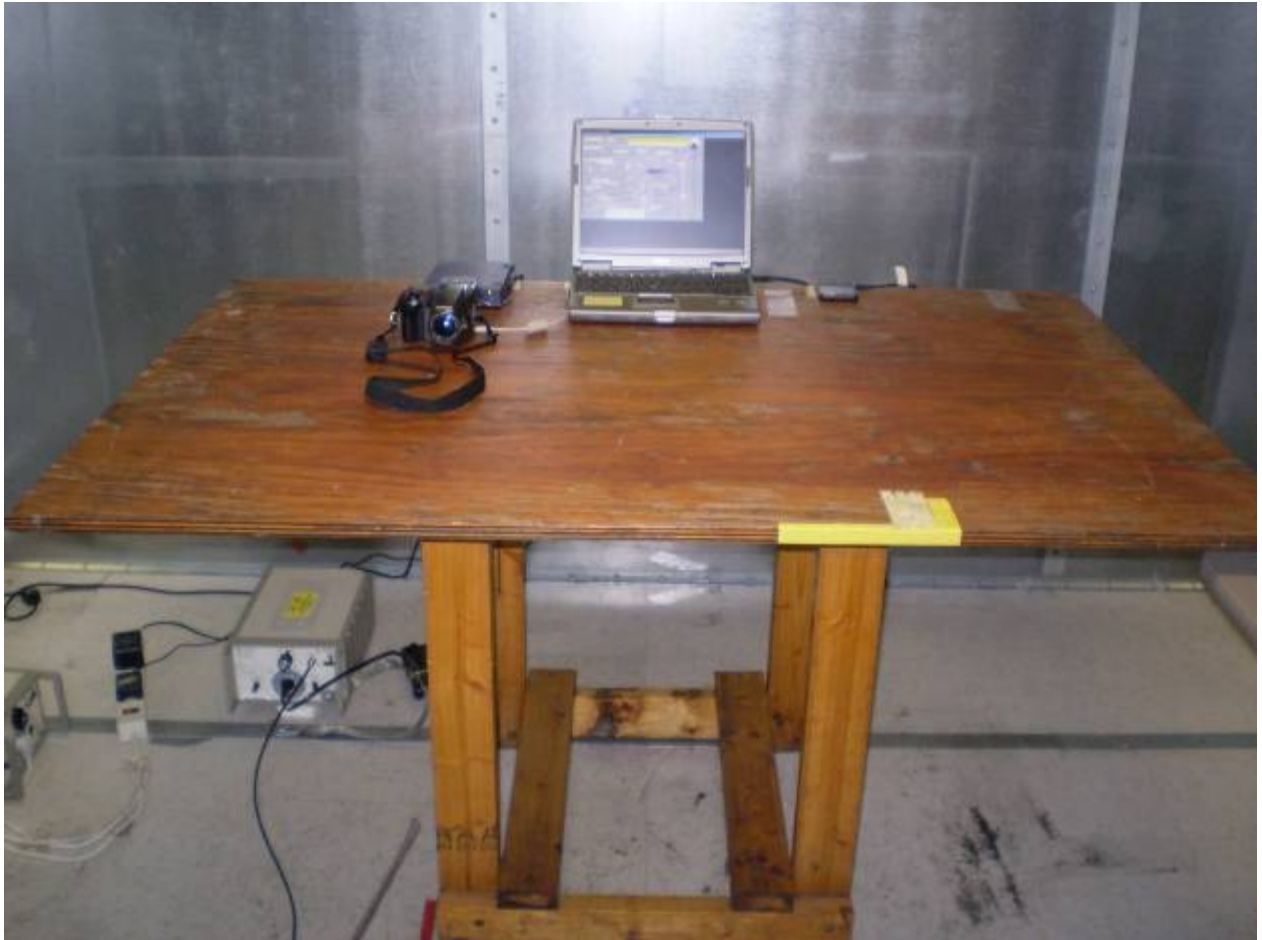
AC Line Conducted Emissions - Part 15 PC Peripheral
