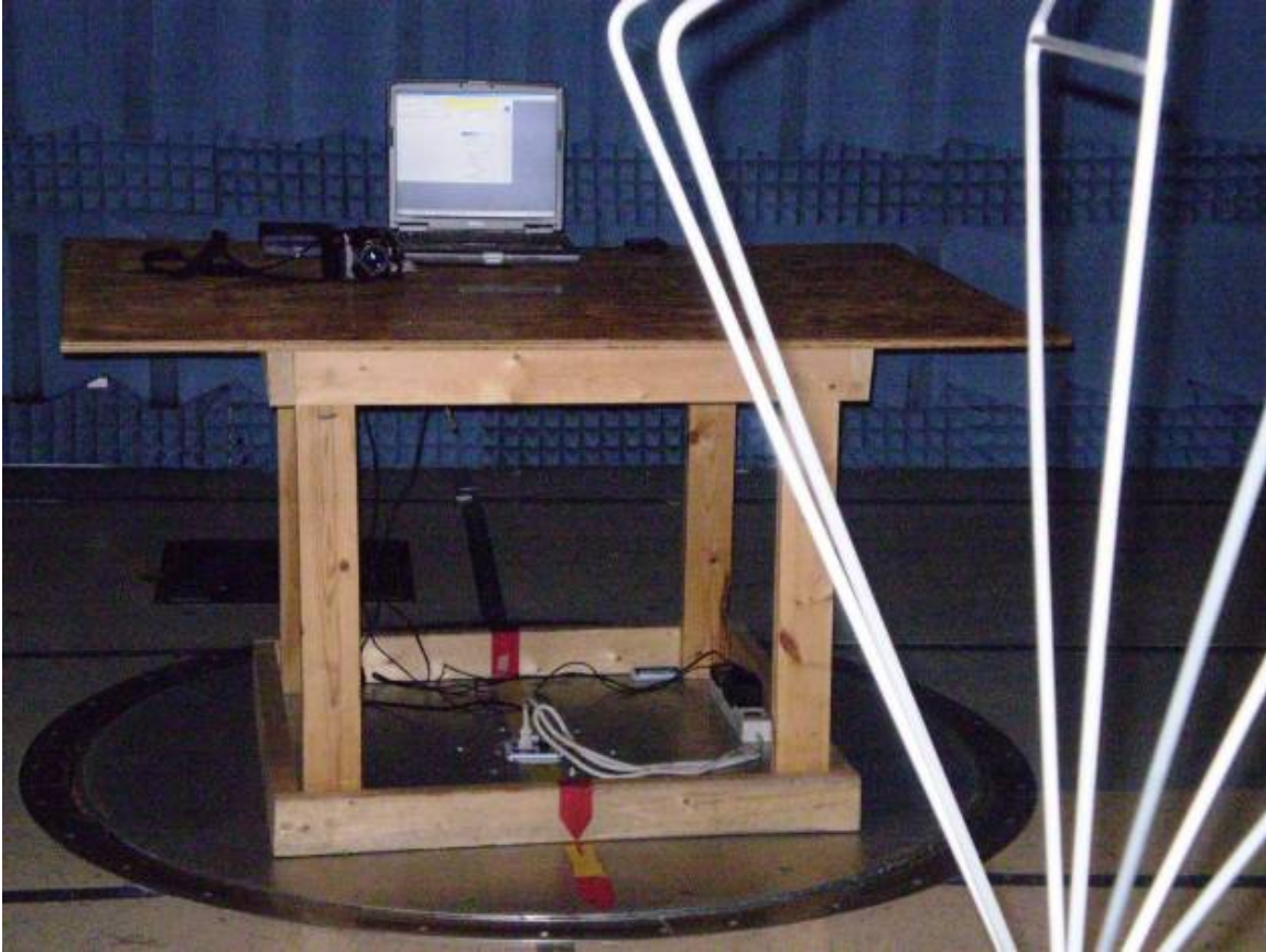
Radiated Emissions - Part 15 PC Peripheral
