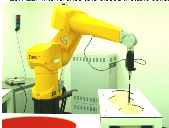
Fig 5.5 Photo of DASY4
