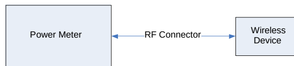
Figure 13-2 Power Measurement Setup
