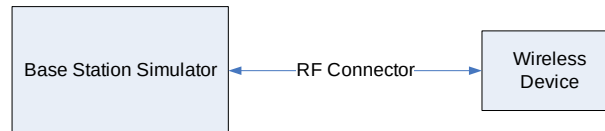
Figure 13-1 Power Measurement Setup
