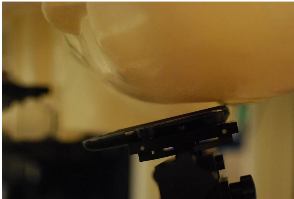
SAR Test Setup Photo 4 – Left Tilt
