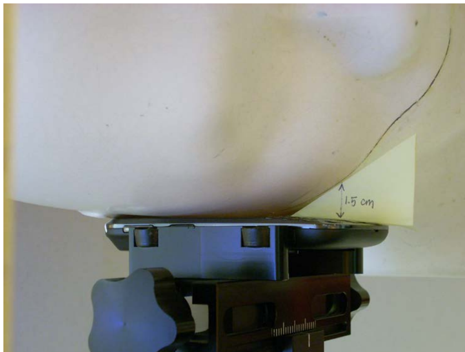
SAR Test Setup Photo 12 – Mouth-Jaw Distance
