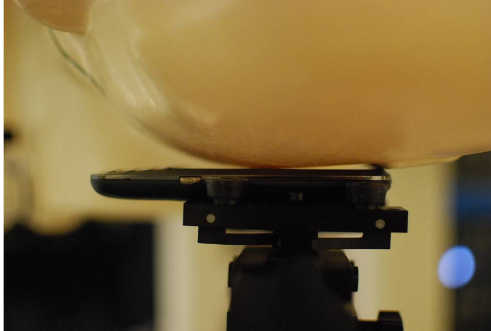
SAR Test Setup Photo 3 – Left Touch
