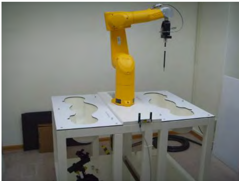
Fig.1 Photograph of the SAR measurement System
