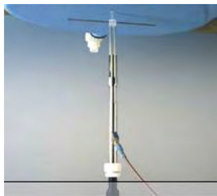
Photograph of the dipole Antenna
