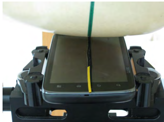
Fig.4 Right Head Section / Ear-Tilt Position(15°)
