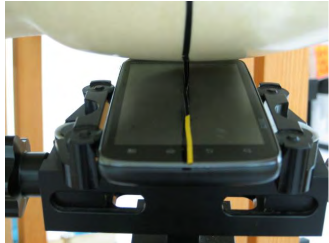
Fig.6 Left Head Section / Ear-Tilt Position(15°)
