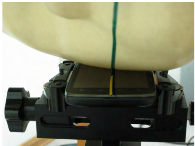
Fig.3 Right Head Section / Cheek-Touch Position
