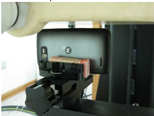
Fig.12 Hotsopt mode- EUT Left to flat phantom and distance between flat phantom and mobile phone is 1 cm.
