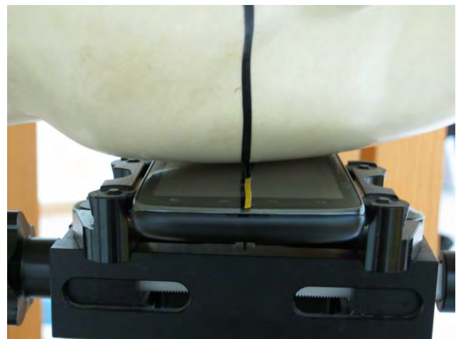
Fig.5 Left Head Section / Cheek-Touch Position
