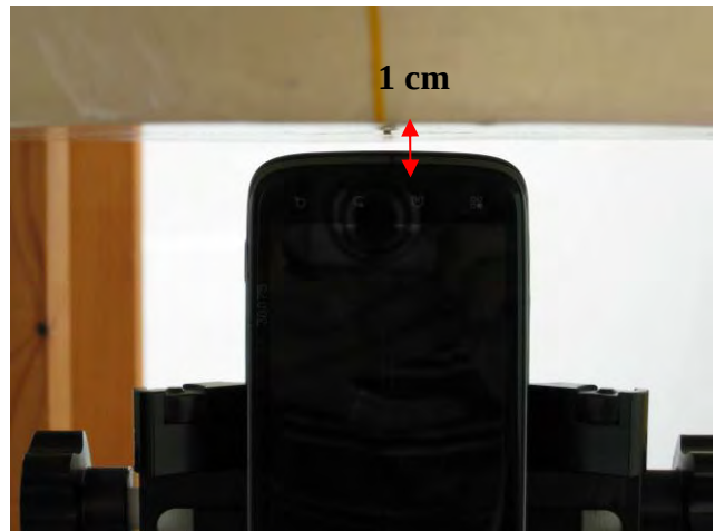
Fig.10 Hotspot mode- EUT Bottom to flat phantom and distance between flat phantom and mobile phone is 1 cm.
