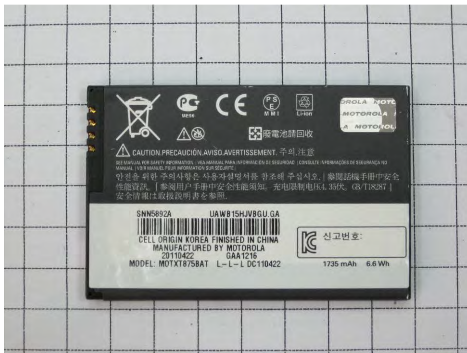
Fig.16 Back view of Battery
