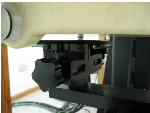
Fig.8 Hotsopt mode- EUT back to flat phantom and distance between flat phantom and mobile phone is 1 cm.
