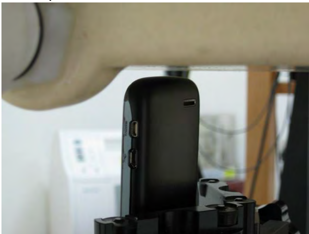
Fig.10 Hotspot mode- EUT Bottom to flat phantom and distance between flat phantom and mobile phone is 1 cm.
