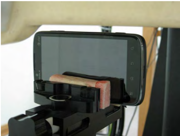
Fig.11 Hotsopt mode- EUT Right to flat phantom and distance between flat phantom and mobile phone is 1 cm.
