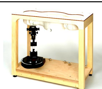
Fig 5.9 Photo of SAM Phantom
