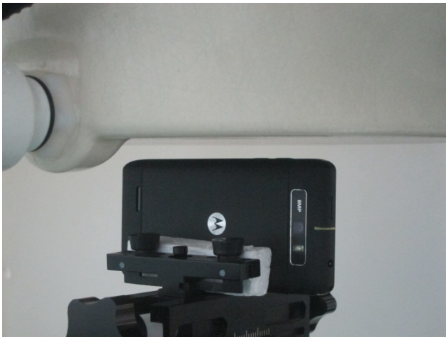
Right Side of the EUT with Phantom 1.0 cm Gap
