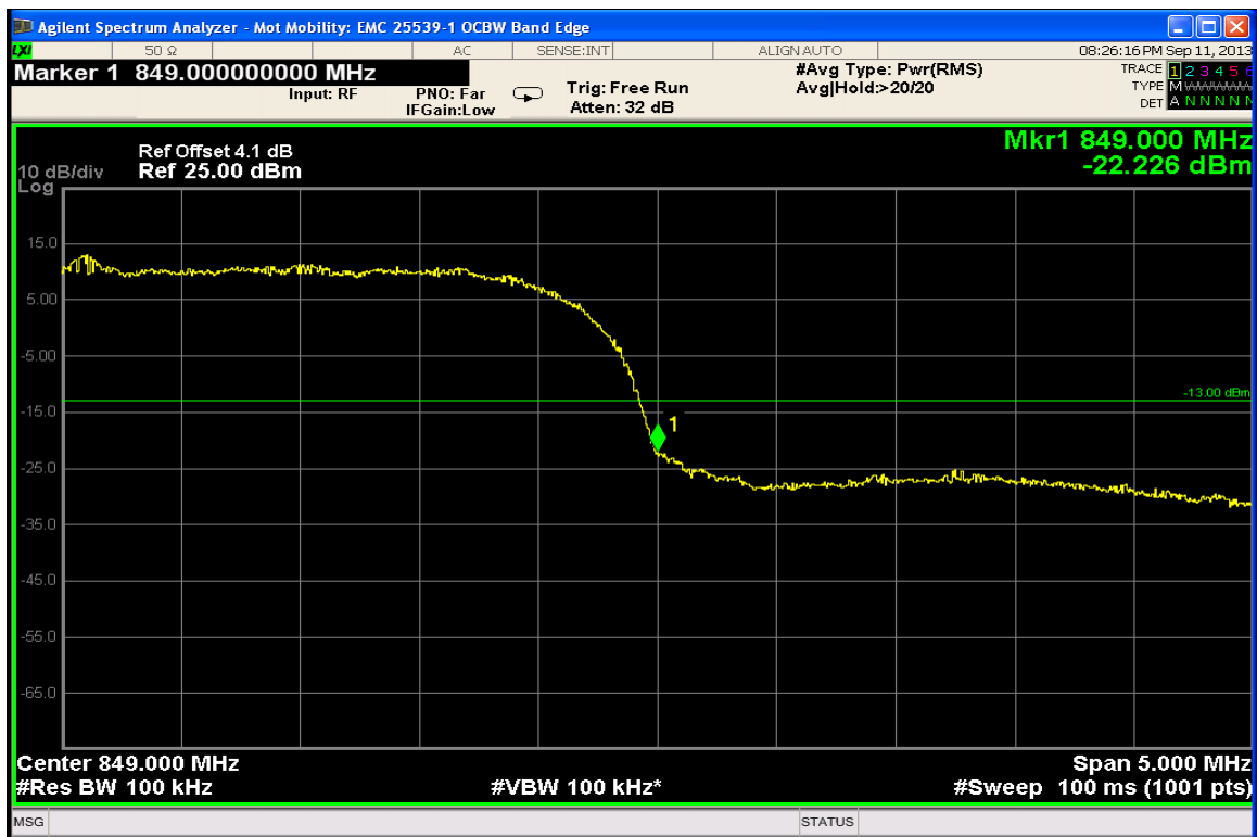
WCDMA 850 – Upper Band Edge – Channel 4233 (846.6 MHz)
