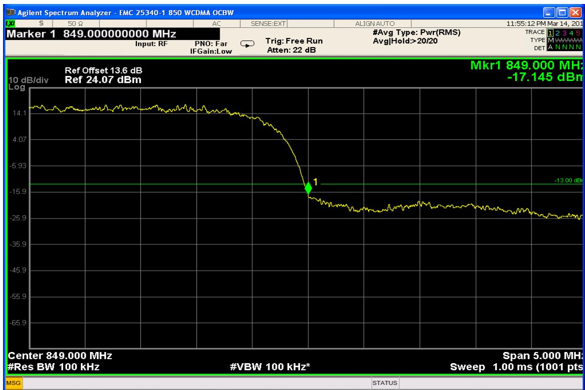
WCDMA 850 – Upper Band Edge – Channel 4233 (846.6 MHz)
