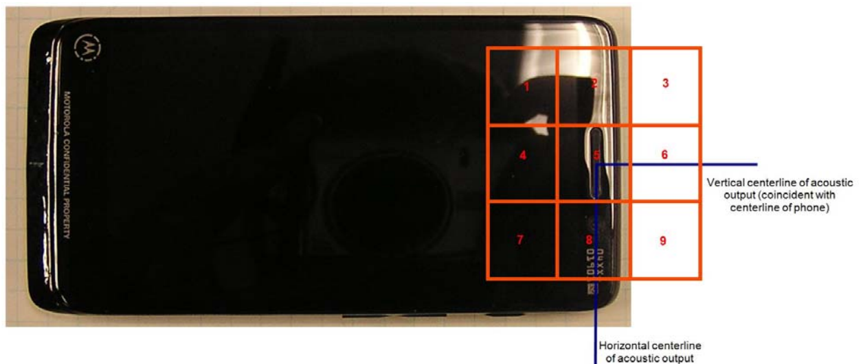
Figure 2. Phone Front - Orientation and Measurement Plane for RF Emissions Testing
