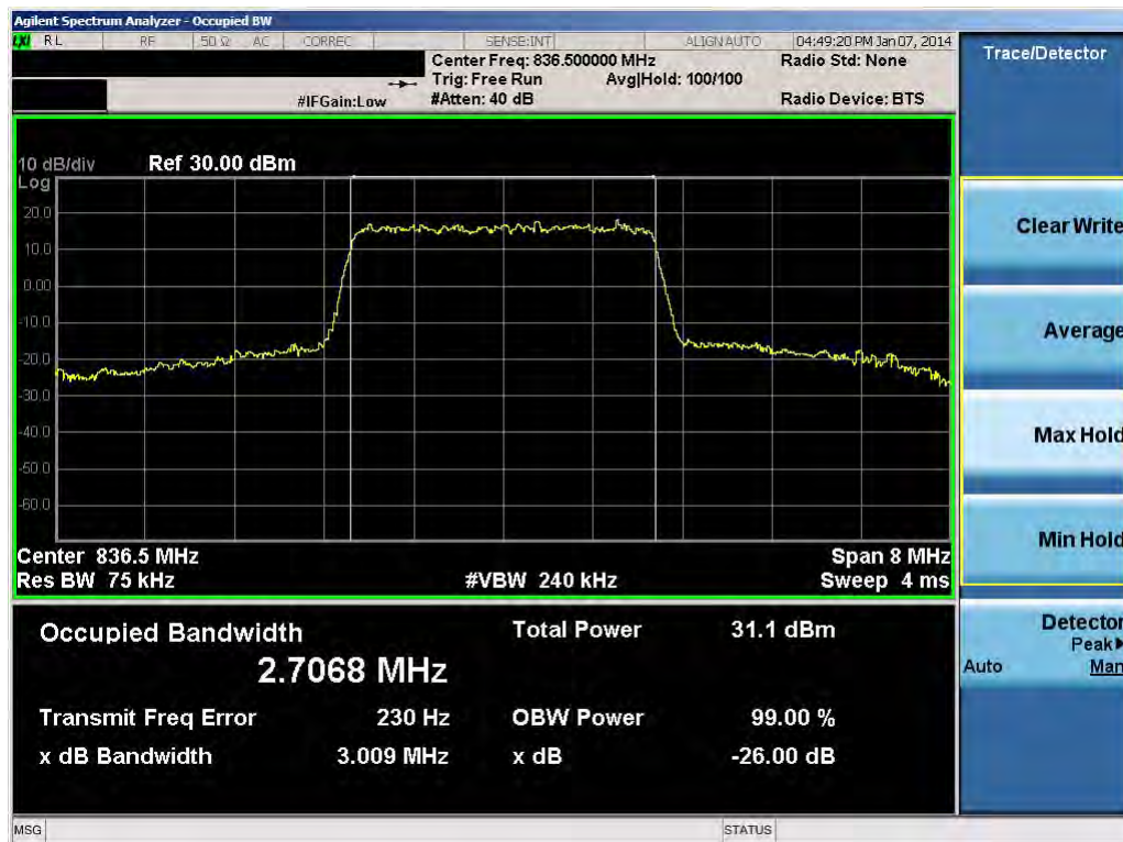
Plot 8-12. Occupied Bandwidth Plot (3.0MHz QPSK – RB Size 15)
