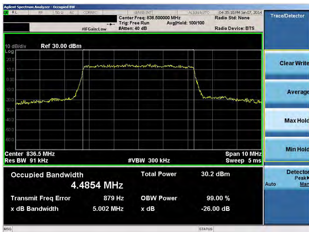
Plot 8-23. Occupied Bandwidth Plot (5.0MHz 16-QAM – RB Size 25)
