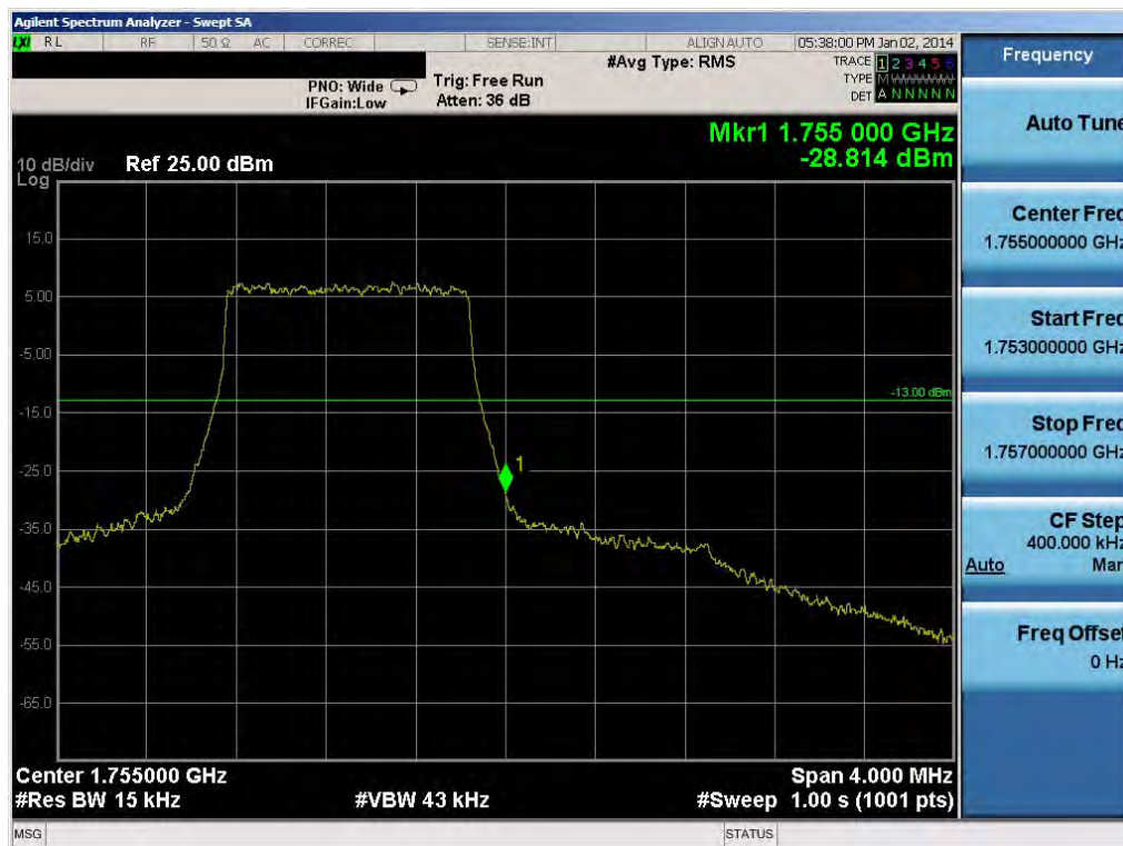
Plot 9-11. Upper Band Edge Plot (1.4MHz QPSK – RB Size 6)
