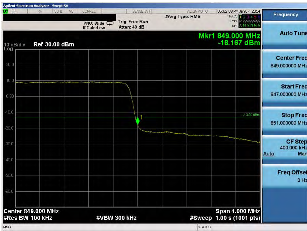
Plot 8-20. Upper Band Edge Plot (3.0MHz QPSK - RB Size 15)
