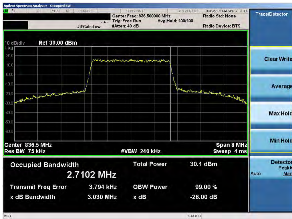
Plot 8-13. Occupied Bandwidth Plot (3.0MHz 16-QAM – RB Size 15)
