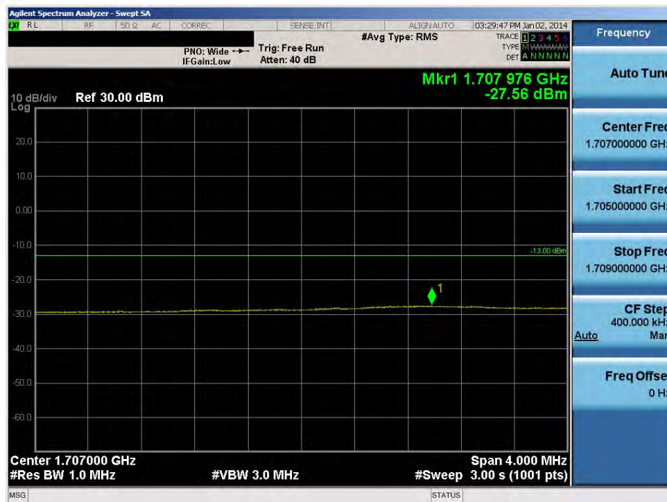
Plot 9-58. Lower Extended Band Edge Plot (15.0MHz QPSK – RB Size 75)
