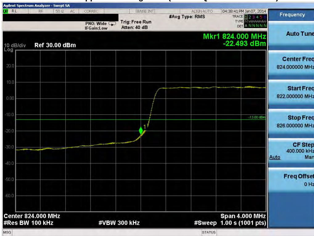
Plot 8-21. Lower Band Edge Plot (5.0MHz QPSK - RB Size 25)
