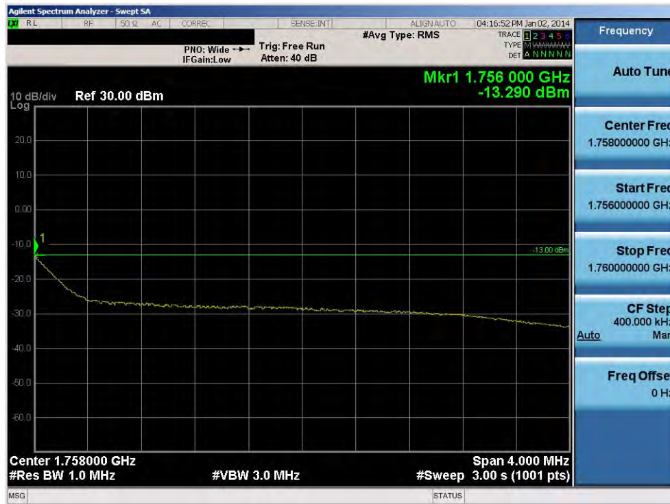
Plot 9-40. Upper Extended Band Edge Plot (5.0MHz QPSK – RB Size 25)
