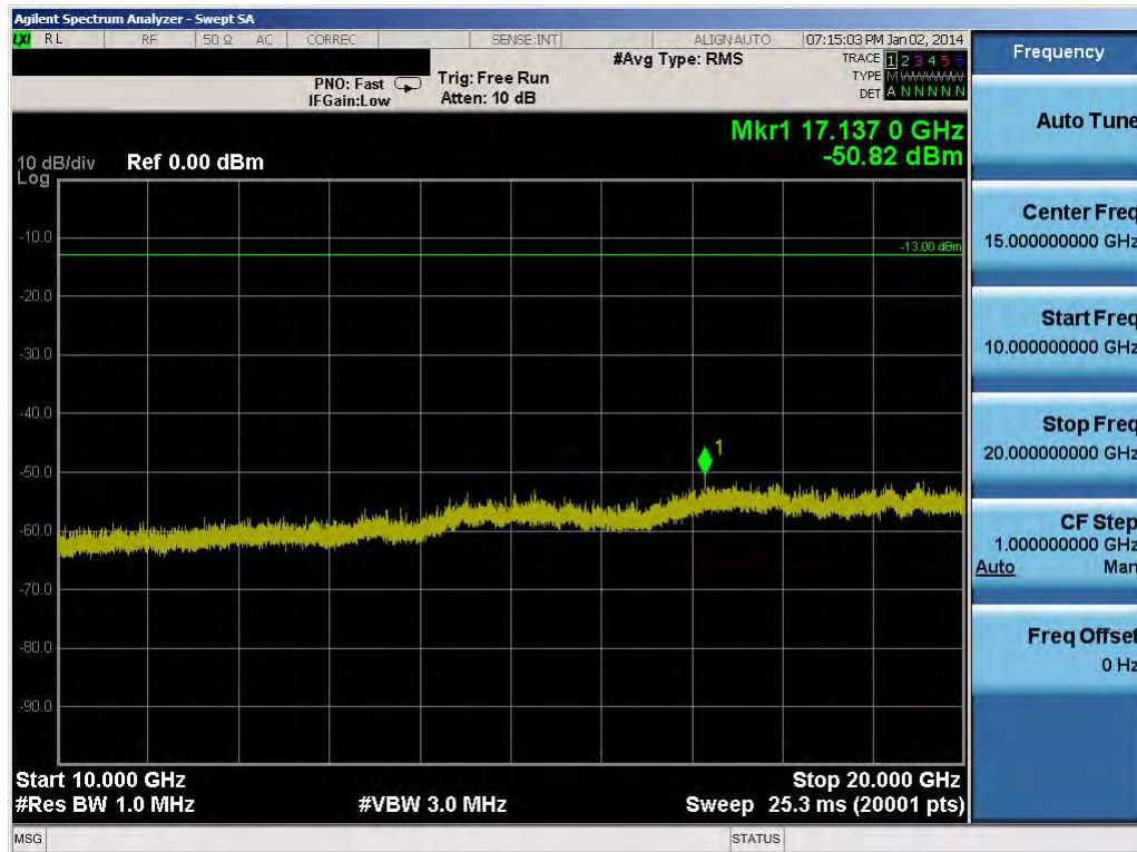
Plot 10-76. Conducted Spurious Plot (20.0MHz QPSK – RB Size 1, RB Offset 0 – Low Channel)
