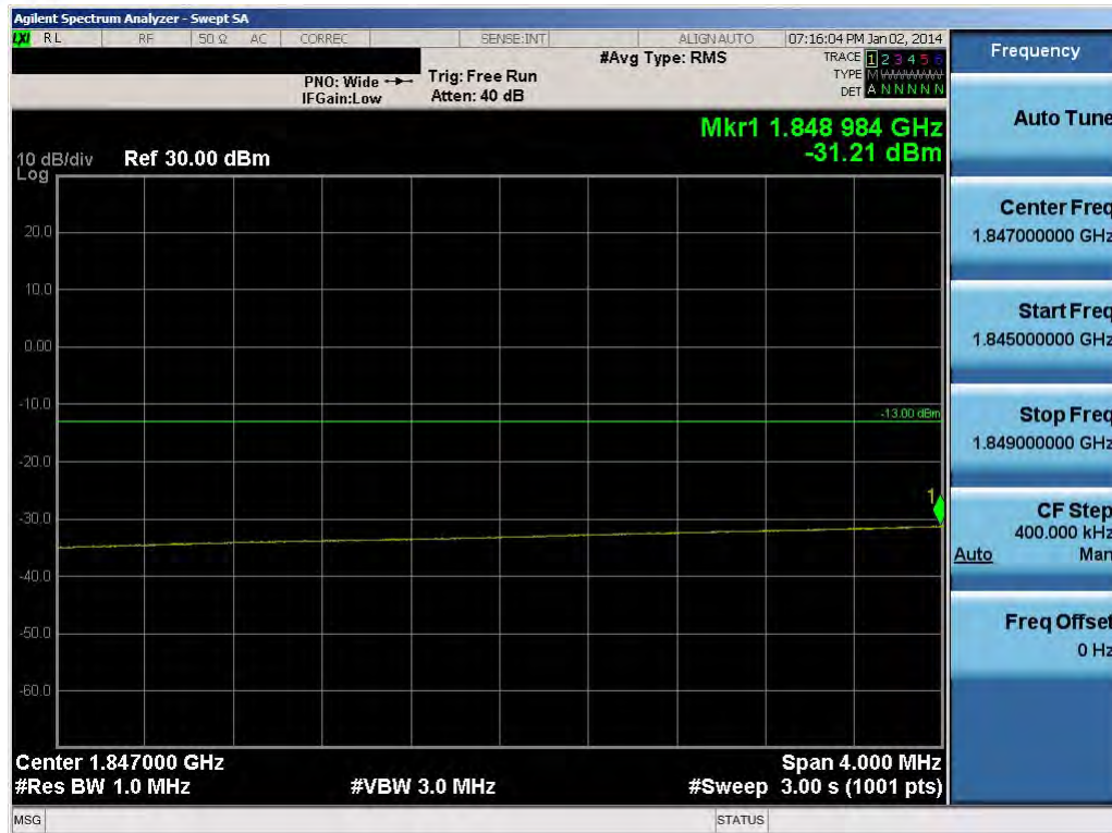
Plot 10-72. Lower Extended Band Edge Plot (20.0MHz QPSK – RB Size 100)
