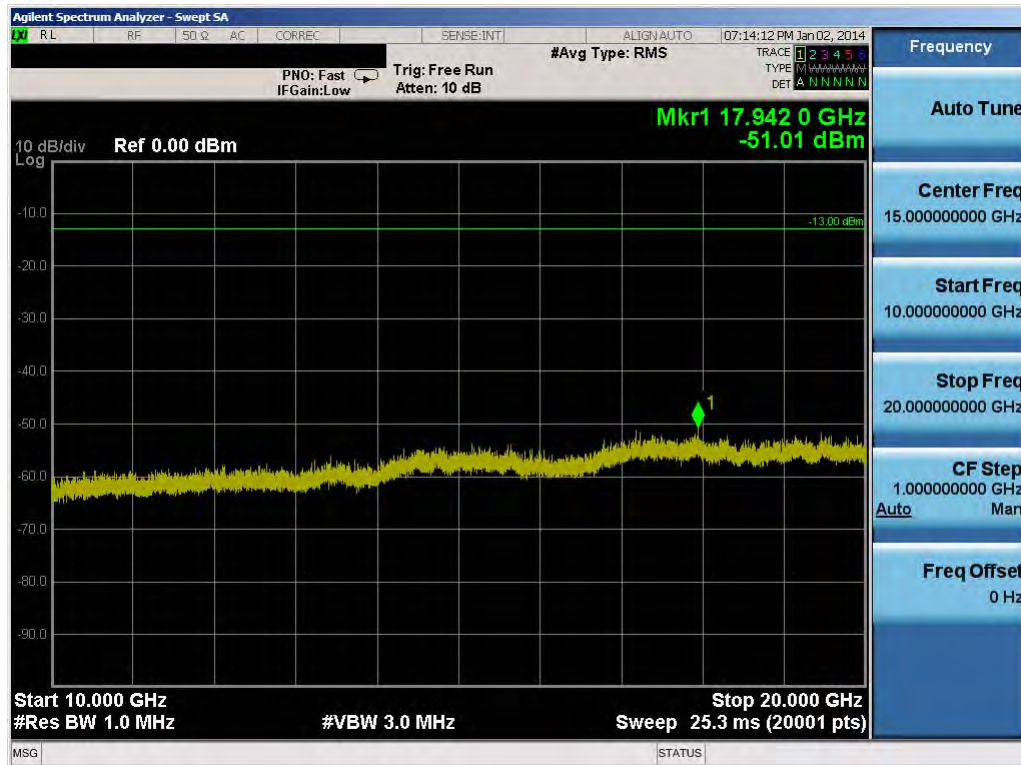
Plot 10-78. Conducted Spurious Plot (20.0MHz QPSK – RB Size 1, RB Offset 0 – Mid Channel)
