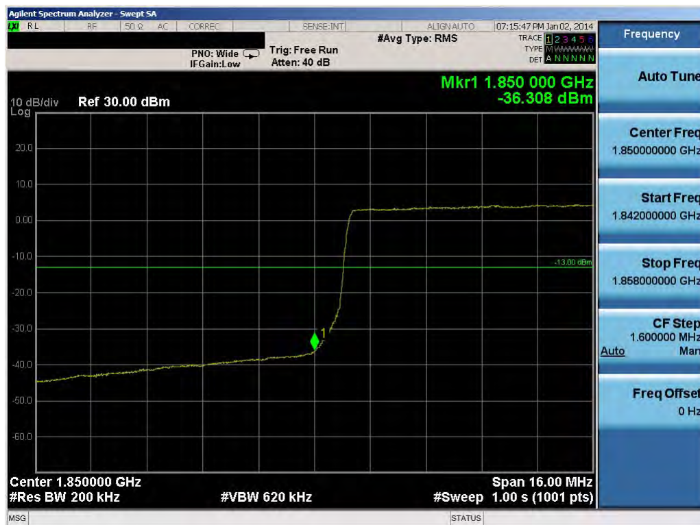
Plot 10-71. Lower Band Edge Plot (20.0MHz QPSK – RB Size 100)
