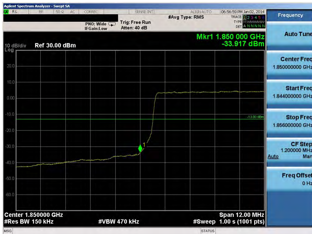
Plot 10-57. Lower Band Edge Plot (15.0MHz QPSK – RB Size 75)
