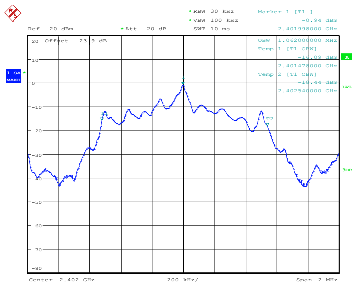
99% Bandwidth Plot on Channel 00
