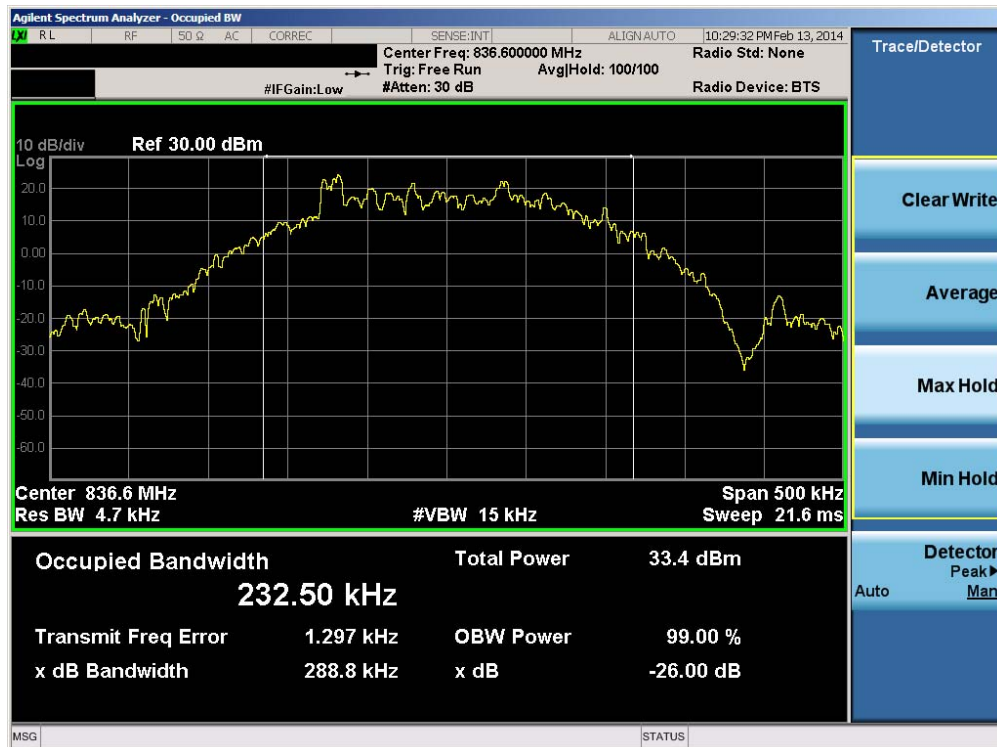
Plot 6-2. Occupied Bandwidth Plot (EDGE850 Mode – Ch. 190)
