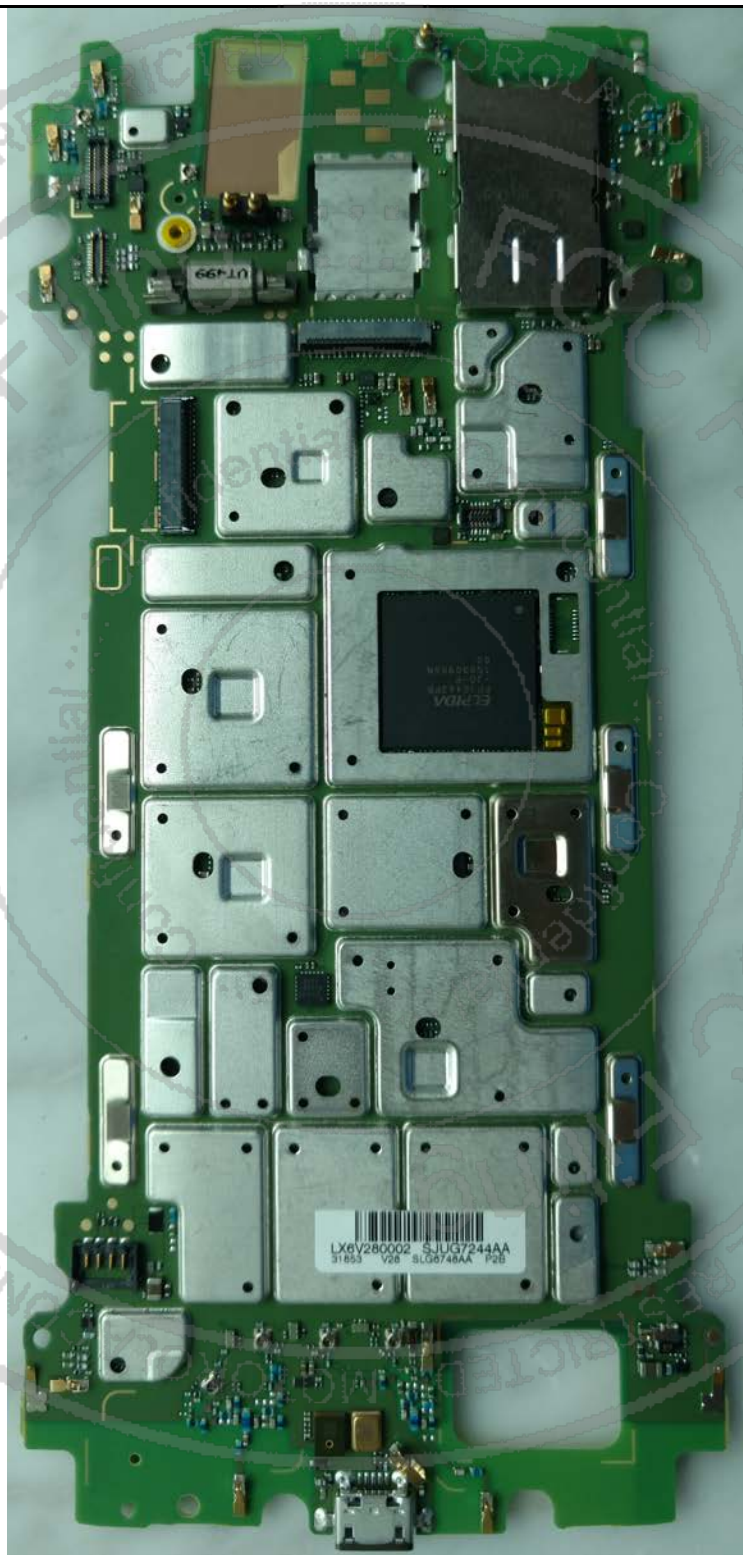
Photograph 9-1: Front side view of the device's PC Board, Shields in place.
