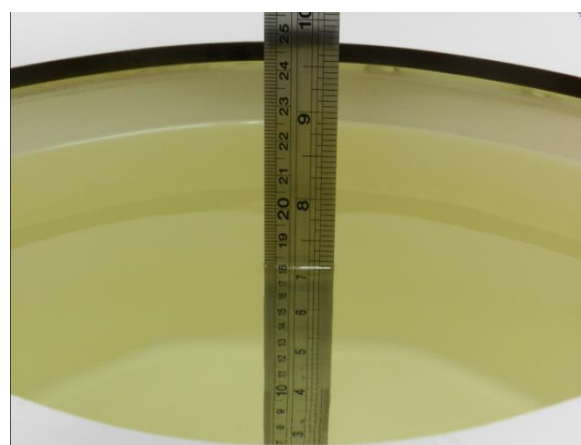
Fig 10.2 Photo of Liquid Height for Body SAR
