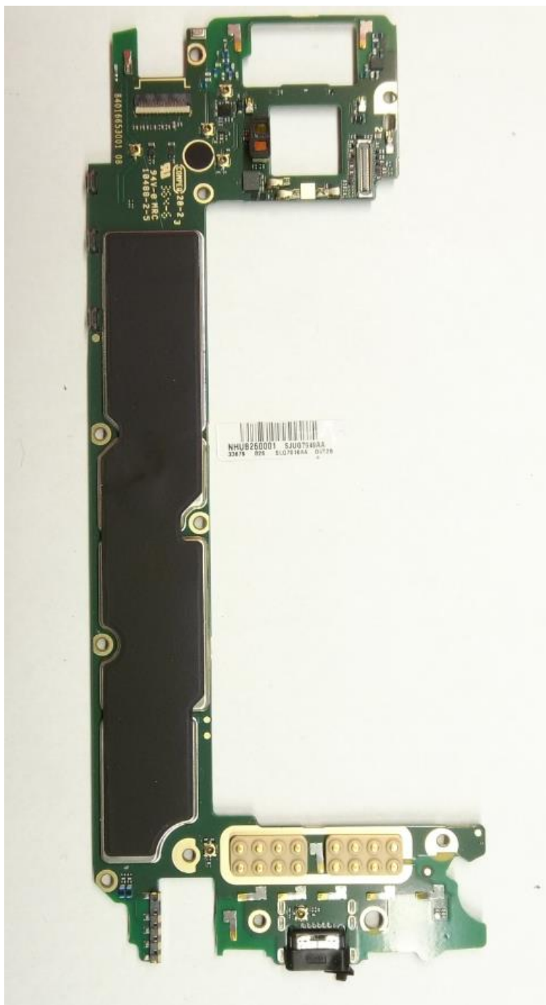
Photograph 9-1: PCB with Shields – Front (Display) Side
