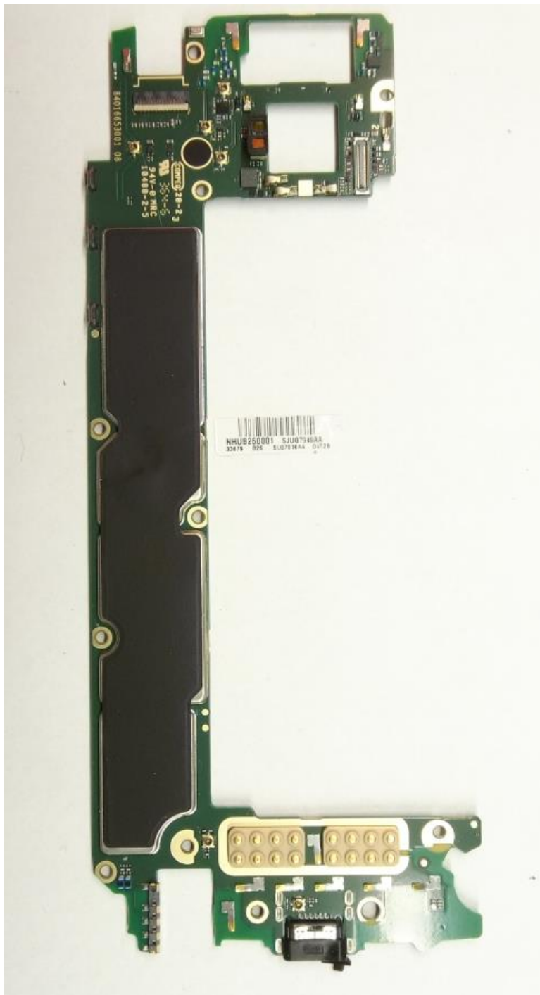
Photograph 9-1: PCB with Shields – Front (Display) Side
