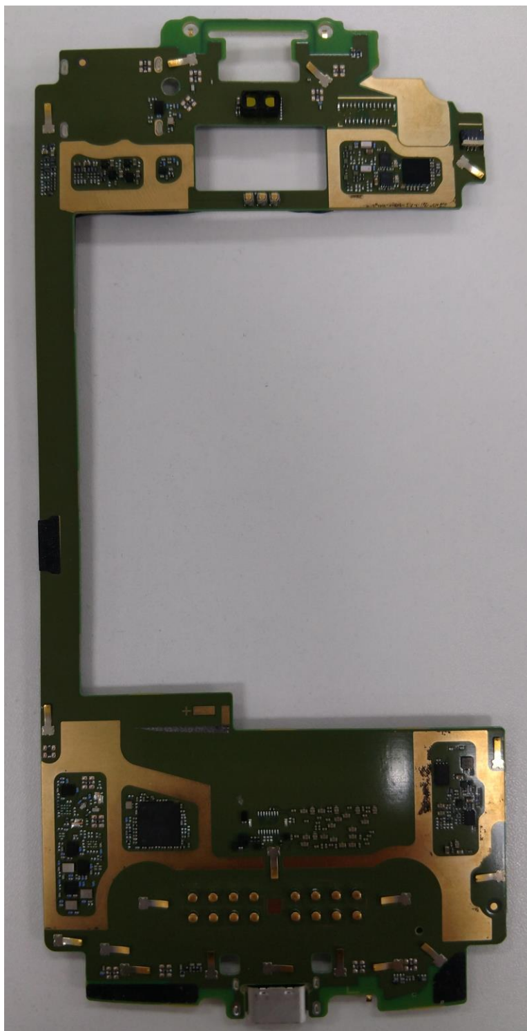
Photograph 9-2: PCB – Back (Battery) Side
