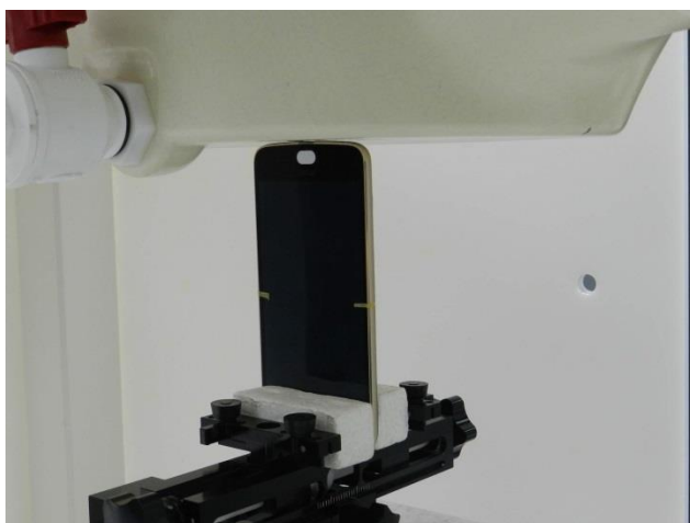
Bottom Side, Test Separation 0 mm
