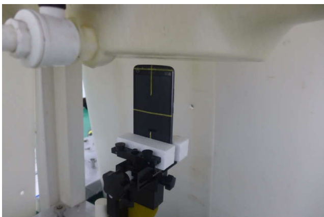
Top Side, Test Separation 10 mm
