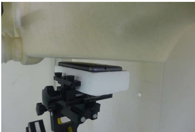
Back, Test Separation 10 mm
