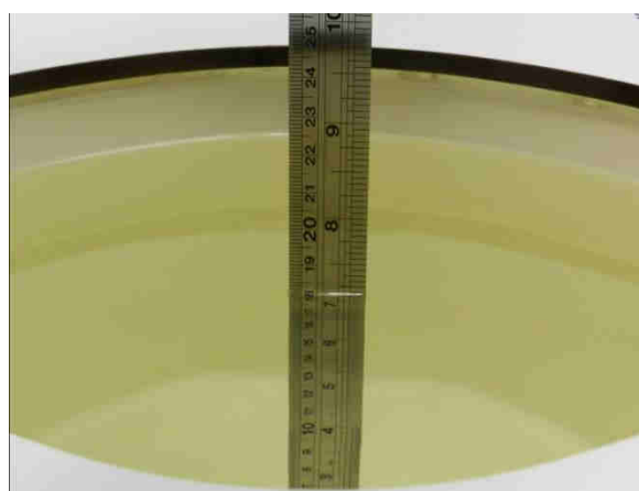
Fig 10.2 Photo of Liquid Height for Body SAR
