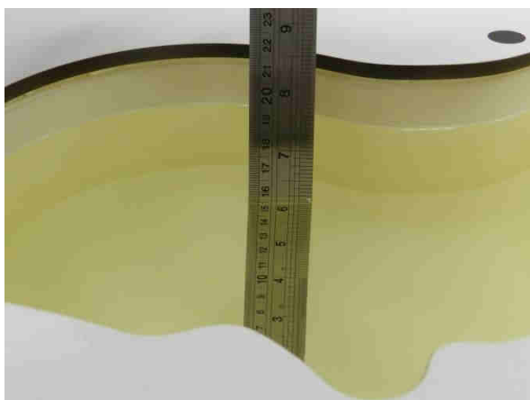
Fig 10.1 Photo of Liquid Height for Head SAR
