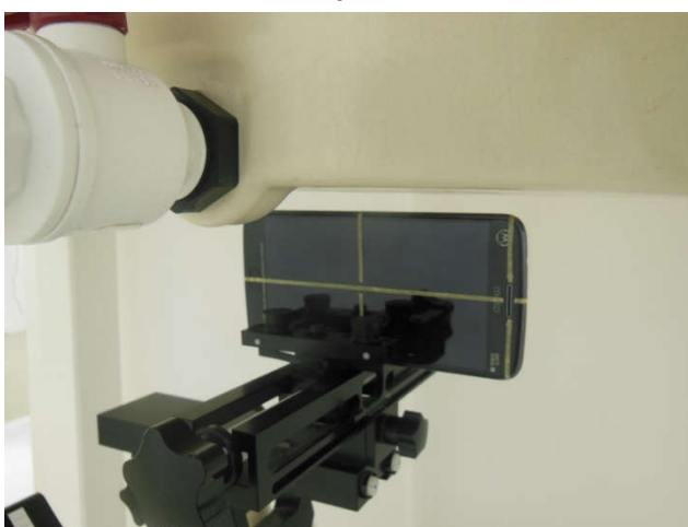
Left Side, Test Separation 10 mm
