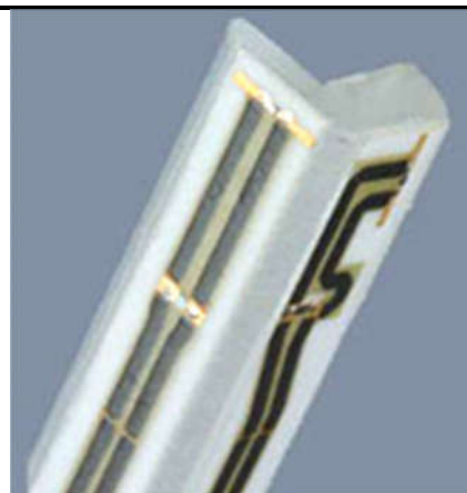
Fig 5.2 Photo of E-field Probe
