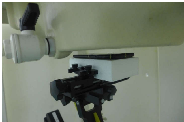
Front, Test Separation 10 mm
