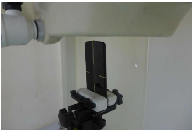
Bottom Side, Test Separation 10 mm
