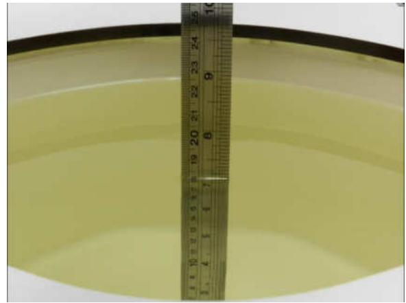
Fig 10.2 Photo of Liquid Height for Body SAR
