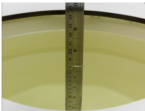
Fig 10.2 Photo of Liquid Height for Body SAR
