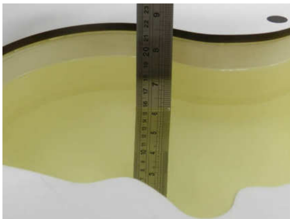
Fig 11.1 Photo of Liquid Height for Head SAR
