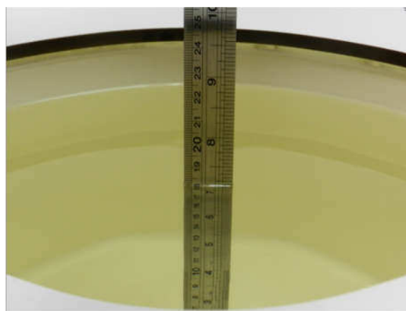
Fig 11.2 Photo of Liquid Height for Body SAR
