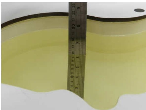
Fig 10.1 Photo of Liquid Height for Head SAR
