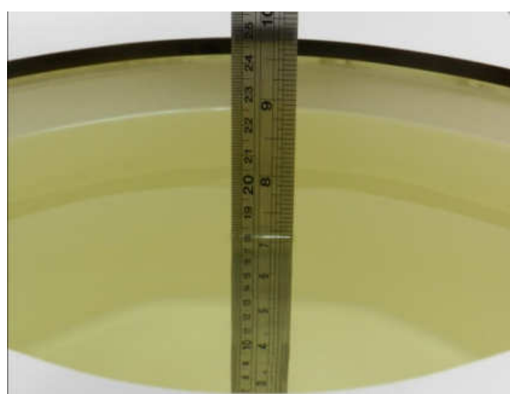
Fig 10.2 Photo of Liquid Height for Body SAR
