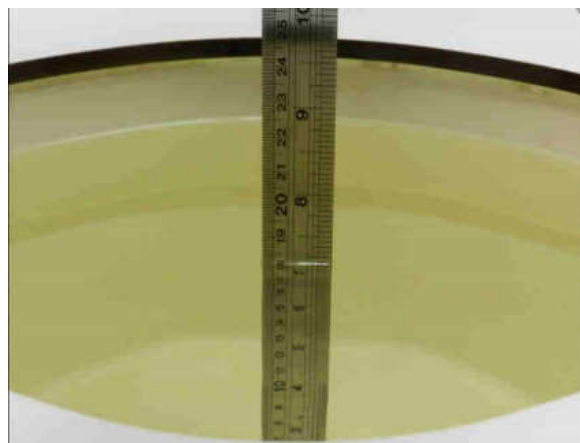
Fig 10.2 Photo of Liquid Height for Body SAR
