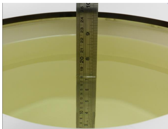
Fig 10.2 Photo of Liquid Height for Body SAR
