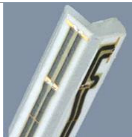
Fig 5.2 Photo of E-field Probe
