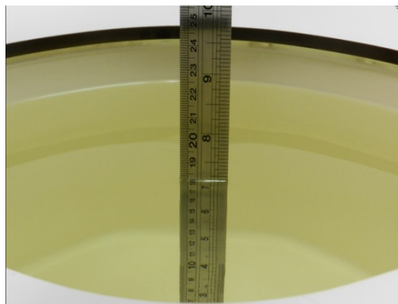
Fig 10.2 Photo of Liquid Height for Body SAR
