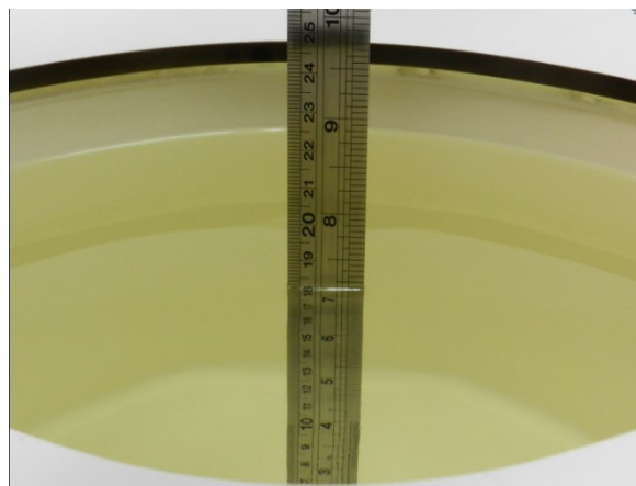
Fig 10.2 Photo of Liquid Height for Body SAR
