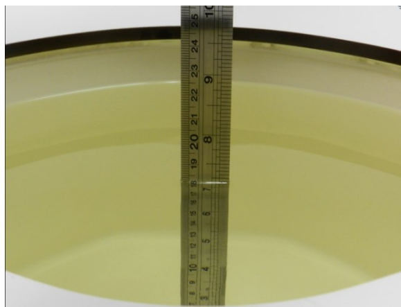
Fig 10.2 Photo of Liquid Height for Body SAR
