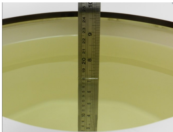
Fig 10.2 Photo of Liquid Height for Body SAR
